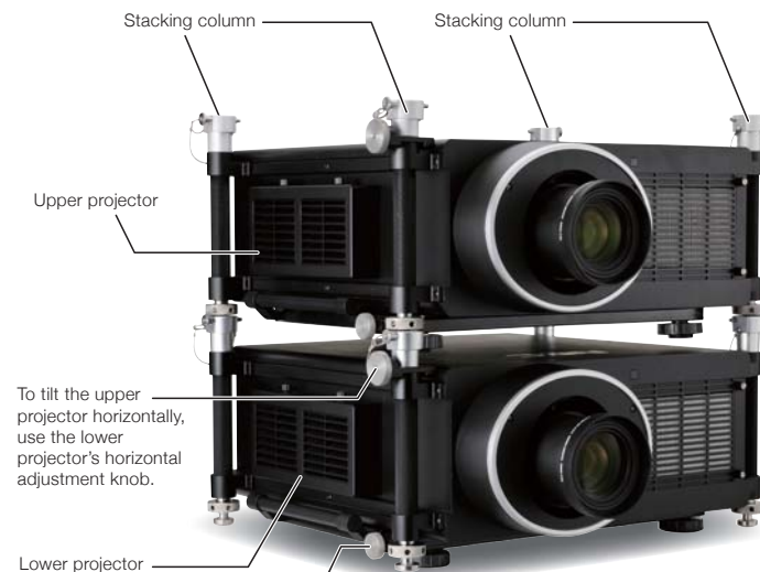
The stacking columns can facilitate not only vertical but also horizontal projection angle adjustment.
